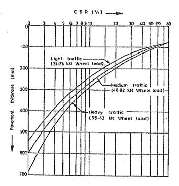
Calculation of sub base course thickness  $(t_{sb})$ : By using the above chart, forgive CBR value of sub base course material and for wheel load read the thickness of pavement which is above the soil sub base. It is denoted as (Tsb). Which is highlighted by circle in the below fig. but here we have to find  $t_{sb}$ . Therefore, thickness of sub base course  $t_{sb} = T - Tsb$
