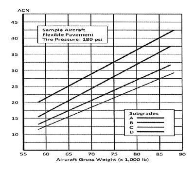
system of classification of the supporting capacity of pavements, indicating their ability to support loads without cracking or becoming permanently deformed.
