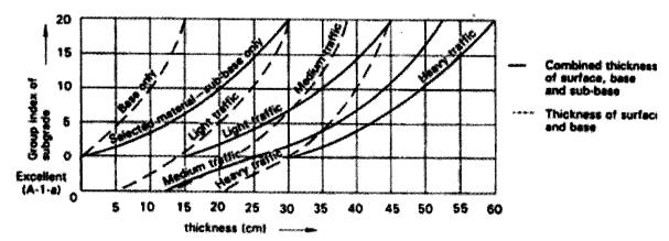
Calculation thickness of sub-base course (t<sub>sb</sub>): From the below chart for given group index of soil subgrade select appropriate curve value of "thickness of sub base only" which will give the thickness of the sub-base course. The curve highlighted in below diagram
