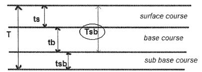
Calculation of base course thickness  $(t_b)$ : Repeat the above procedure again, from the CBR value of base course and from traffic intensity value read the value of thickness of pavement which is above the base course  $(t_s)$ . From this we can find out the value of  $t_b$ .  $t_b = T_{sb} - t_s$  Therefore all the values of pavement are known and cross section of pavement is as follows.
