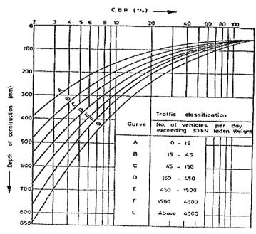
Calculation of sub base course thickness ( $t_{sb}$ ): By using the above chart, for give CBR value of sub base course material and for traffic intensity value read the thickness of pavement which is above the soil sub base. It is denoted as (Tsb). Which is highlighted by circle in the below fig. but here we have to find  $t_{sb}$ . Therefore, thickness of sub base course  $t_{sb} = T - Tsb$
