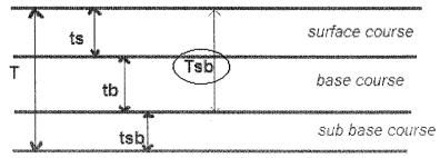
Calculation of base course thickness ( $t_b$ ): Similar to the above procedure, from the CBR value of base course and wheel load read the value of thickness of pavement which is above the base
