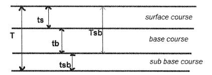
CBR method recommended by IRC (Indian road congress): In this method, the chart contains several curves (A, B, C, D, E, F, and G) which represents the different levels of traffic intensities. Based on this we will find out the layers thicknesses.
