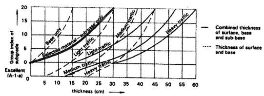
Calculation of thickness of base and surface course ( $t_b$  &  $t_s$ ): Thickness of surface and base course = total thickness – sub-base thickness =  $T - t_{sb}$  The combined value of thickness of base and surface course can be found out from above chart form dotted curve with the help of group index value and traffic volume. Or otherwise assume the thickness of surface course ( $t_s$ ) = 5 cm Then we can easily calculate the value of thickness of the base course,
