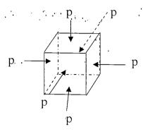
. Volumetric stress produces a change in volume of the body without producing any distortion to the shape of the body.
