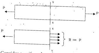
Consider a uniform bar of cross sectional area A subjected to an axial tensile force P. The stress at any section x-x normal to the line of action of the tensile force P is specifically called tensile stress. Since internal resistance R at x-x is equal to the applied force P, we have,
