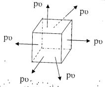
Consider a cube element subjected to volumetric tensile stress  $\sigma v$  in X, Y and Zdirections. Stress in each direction is equal to pv. ie  $\sigma x = \sigma y = \sigma z = \sigma v$
