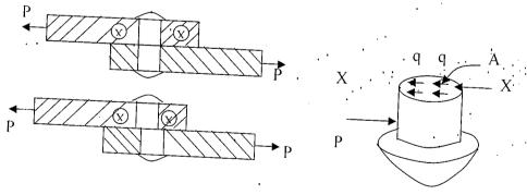
The stresses set up at the section x-x acts along the surface of the section, that is, along a direction tangential to the section. It is specifically called shear or tangential stress at the section and is denoted by q.
