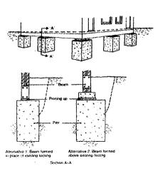
requires that a mini-pile must be installed on either side of the affected wall. After the piles have been installed, then brickwork is removed below the wall and reinforced concrete needle beam is used to connect the piles and support the wall.
