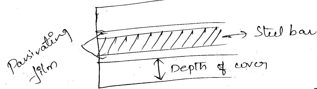
When carbonation occurs the pH get reduced and the alkalinity get reduced, this causes the destruction of Passivating film and water & oxygen reaches it and causes rust.
