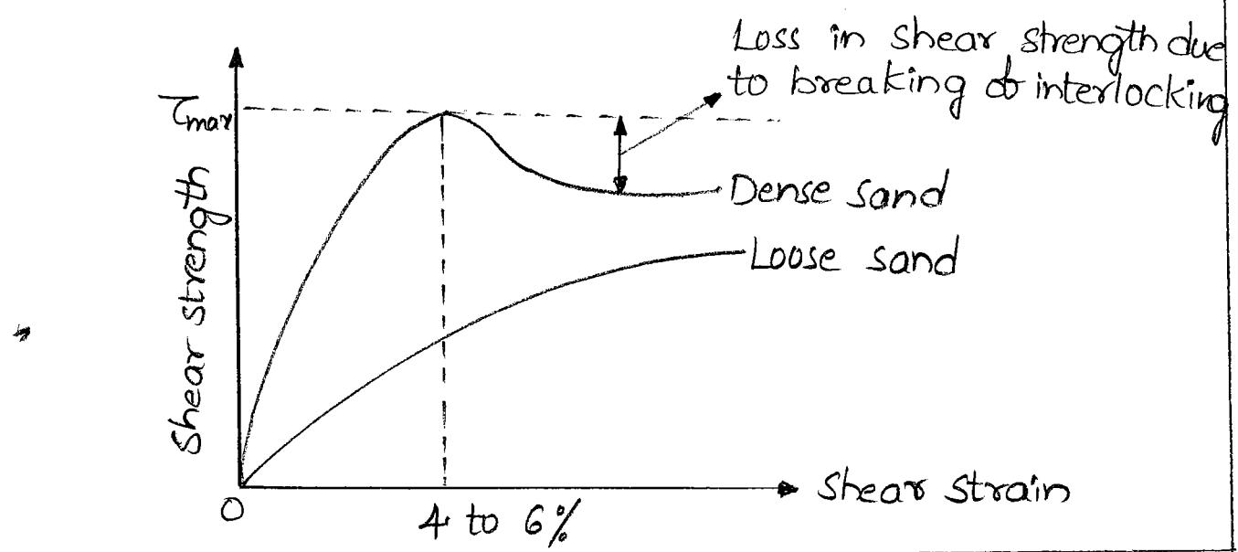
The shear strength of sand is due to
