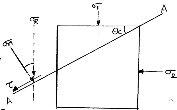
→ On the plane of  $\theta_c$  (critical plane),  $\sigma_R$  is most inclined [i.e.  $\beta = \beta_{max}$ ] for frictional soils  $\beta_{max} \approx$  internal frictional angle of soil ( $\phi$ ).
